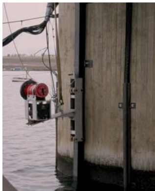
Figure 2.6. Photographs of ADCP/DIDSON Deployment at McNary Dam, 2007
